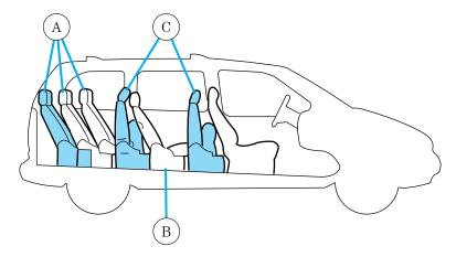
The entire seat can be moved to four seating positions and two storage positions.
